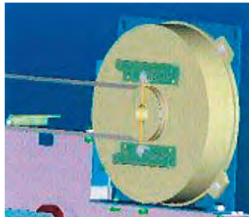
PM motor with VVVF door control (By 3D modeling)
