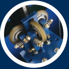
Low friction rollers For superior ride and improved overall comfort
